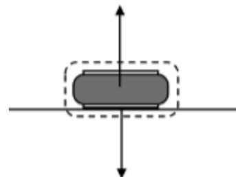
*What happens to the force diagram if the fan is now turned to the on position?* If the surface on which the puck is placed is truly level, the puck will hover motionless on a cushion of air. The gravitational force,  $\vec{F}_g \text{ by } E \text{ on } p$ , will not change. The air instead of the table now provides the upward force. This new force, the upward push on the puck by the air is denoted  $\vec{F}_A \text{ by } a \text{ on } p$ .
