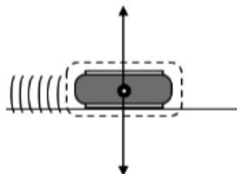
The most important thing to understand about this situation is that the puck will, as long as the forces remain balanced, travel at the same speed in a straight line. Nothing is required to cause the puck to keep moving. An unbalanced force would be required to cause it to go faster or slower, and/or an unbalanced force would be necessary to change its direction. But in the absence of an unbalanced force, the puck will continue to move in a straight line at a constant speed.
