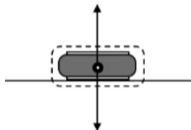
The force diagram looks exactly the same as before, except for the label on the upward force. The unbalanced force on the puck is zero, just as it was when the puck was resting on the table with the fan turned off.
