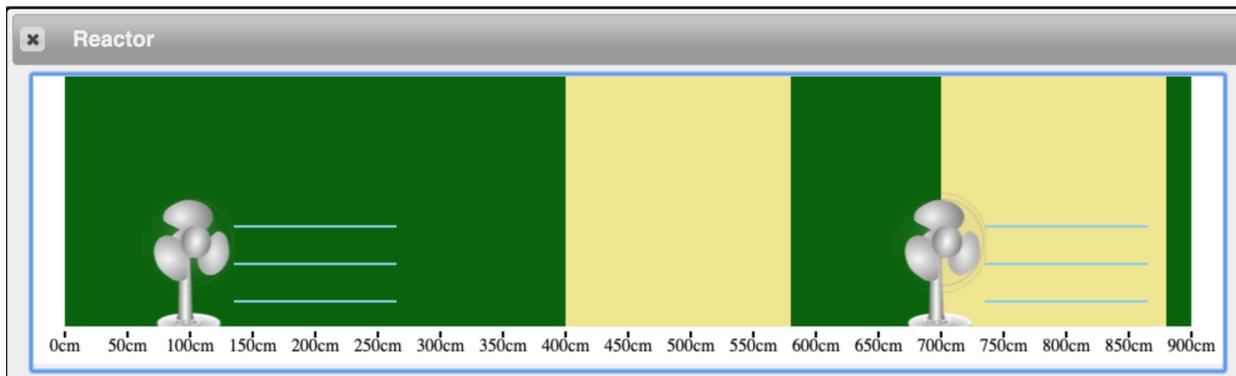
In this simulation a ball moves across the screen with some initial positive velocity. When it is in the area marked with three lines (between 100 cm and 280 cm, and between 700 cm and 880 cm) the wind from the fan gives it an applied force to the right. When it is in the lighter-colored areas (between 400 and 580 cm, and between 700 and 880 cm), there is a resistive force from the sand.
